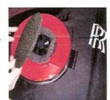
Push fan and filter forward from rear as shown
