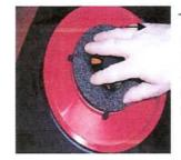
Check the reverse side. The filter should be flush with the surface
